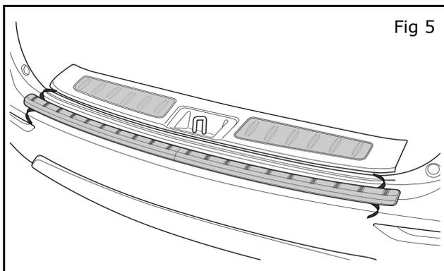
3) Dry fit the bumper protector on the vehicle by aligning the bumper protector centering arrow with the tailgate latch. (Fig 2)
